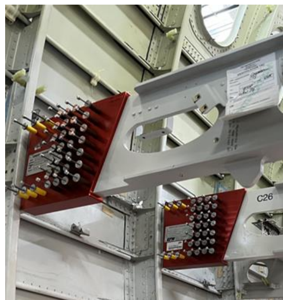
Temporary connection of new and old cross beams
